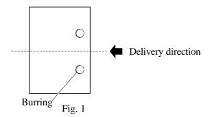
Rear burring is where there is burring at the rear of the punch hole in relation to the direction in which the hole is made.
